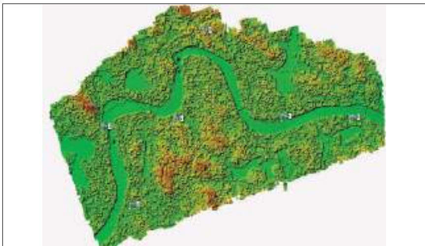
Fig:3.9.Digital Surface Model
