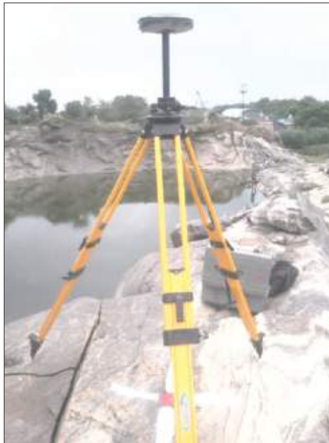
Fig:3.4.DGPS Instrument for GCP Measurement
